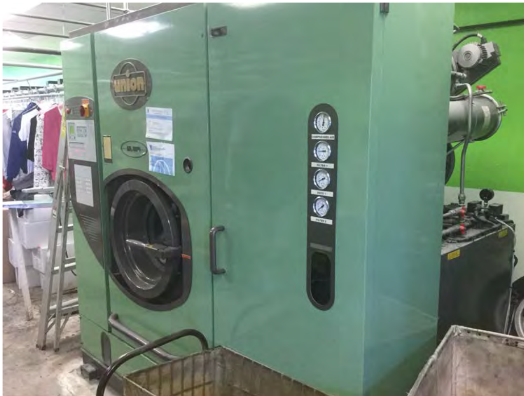
Closed-loop Union HL860 dry cleaning machine. 16285 San Fernando Mission Blvd., Granada Hills, 91344
